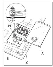
Fig. 6 Connecting the power supply cable-CE604 models
